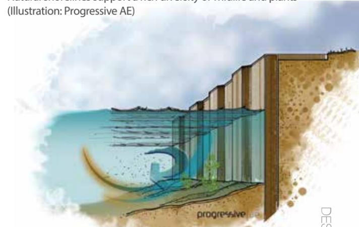
Wave energy transferred downward off a seawall scours the near shore floor of the lake, disturbing the soil and aquatic plants. (Illustration: Progressive AE)
